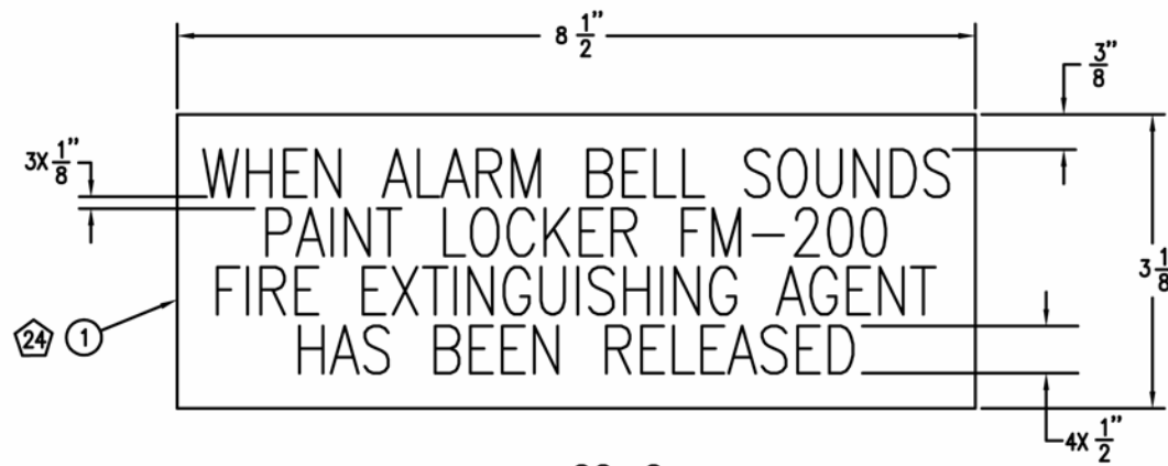
VIEW 22-C PAINT LOCKER FM-200 SYSTEM ALARM BELL LABEL PLATE
