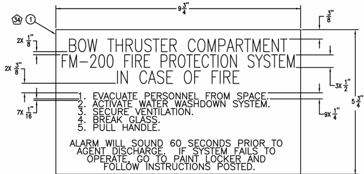
VIEW 46-C BOW THRUSTER COMPARTMENT FM-200 SYSTEM REMOTE OPERATION INSTRUCTION PLATE (A)
